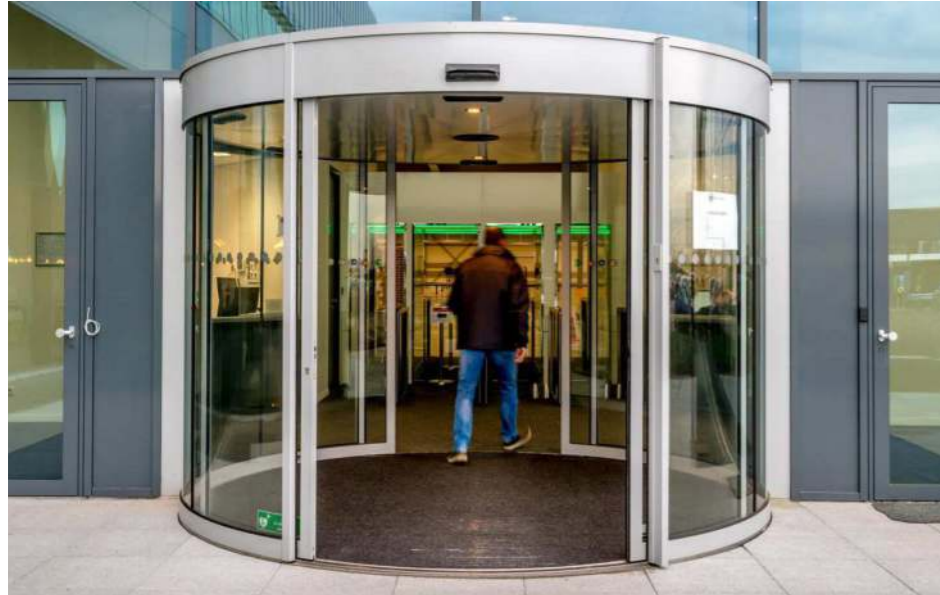
Figure 117 Proposed type of entrance door to provide draught control and accessibility for wheelchair users and those carrying bulky equipment
