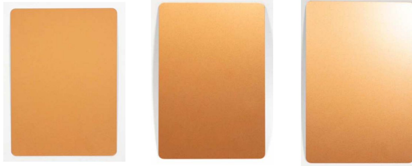
Figure 164 Proposed cladding material sample - PVDF aluminium shingles. Reference photos taken from several lighting angles
